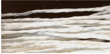
Cocoons are soaked in warm water to soften the gummy sericin. The silken strand from a single cocoon is too fine to use alone, so individual filaments of 6-20 cocoons are unraveled at the same time, traveling through a very small eye. The softened sericin dries, hardens and binds the strands together to become one thread the size of a human hair. It takes many cocoons to make a yarn as thick as the #0.
