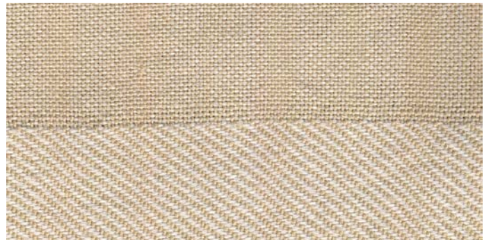
120/8 Tussah Silk warp with 60/4 Silk/Wool (30%/70%) weft in 4 Shaft Plain Weave and Twill, sett 32epi
