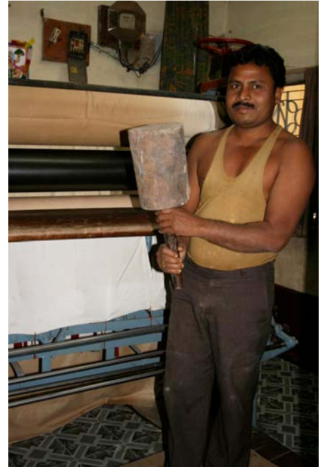
Calendaring machine and an old fashioned mallet used to beat the silk
