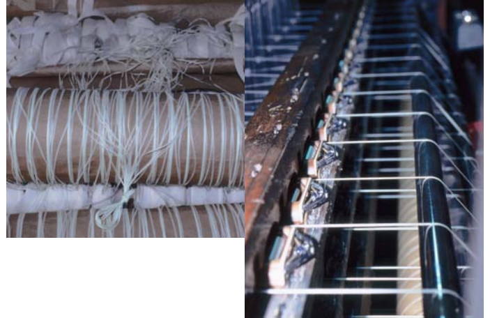
Warp: 8/2 Reeled Silk Weft: Silk Chenille 8 Shaft Block Twill, Sett 22 epi
