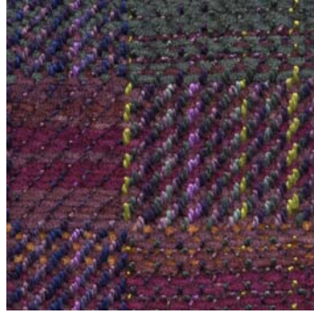
Warp: 8/2 Reeled Silk Weft: Silk Chenille 8 Shaft Block Twill, Sett 22 epi
