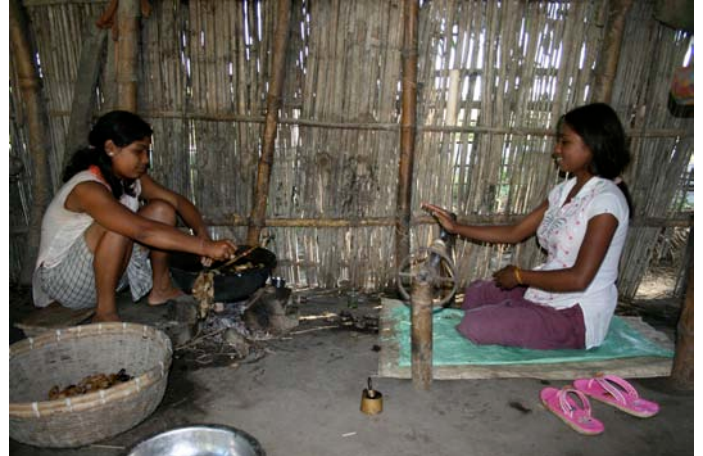
Feeder and reeler on either side of the bhir reeling machine.
